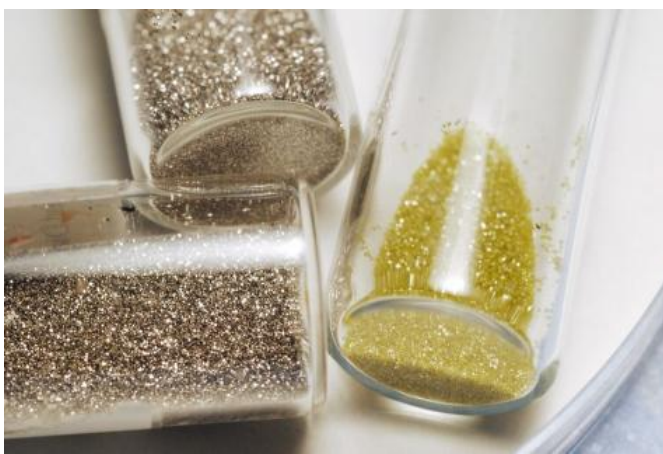
This image shows different preparations of diamonds, ready for integration into a silver matrix. (Credit: Gary Meek)
