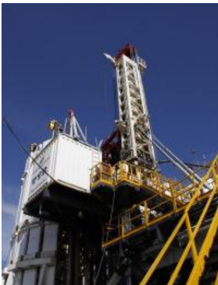
This is the Iceland Drilling Company rig at the Krafla geothermal field, in northern Iceland, that drilled into 900 C rhyolite magma at 2,140 meters depth in June 2009. Credit: W. Elders, UC Riverside.
