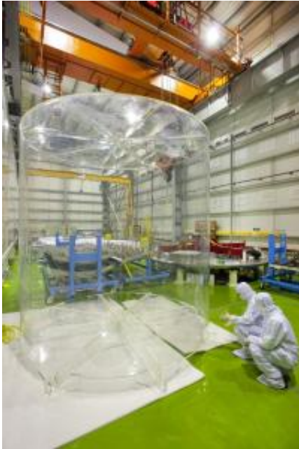
The building where the detectors are assembled is a class 1000 clean room; dust and even microscopic particles in the air are severely limited.
