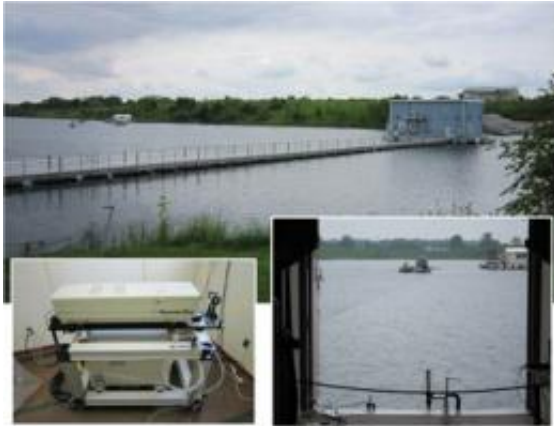
Housed in a floating structure, the Nd:YAG laser (bottom left) generates underwater acoustic pulses, which travel to a distant hydrophone equipped boat (bottom right). Credit: U.S. Naval Research Laboratory (2010)
