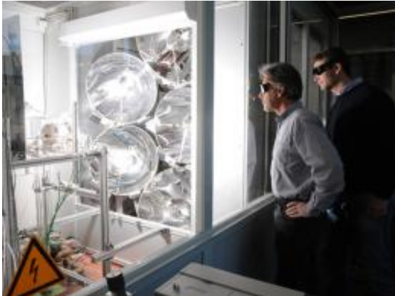
Doctoral student Philipp Furler and Professor Aldo Steinfeld during the experimental investigation of the solar thermochemical reactor under (simulated) concentrated solar radiation. Credit: P. Rüegg / ETH Zurich
