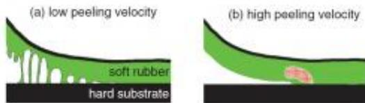
Peeling at low velocity results in a rough surface, while peeling at high velocity results in a smoother surface. Scientists found that both surfaces exhibit unexpected fractal scaling properties. Image credit: B. N. J Persson, et al.
