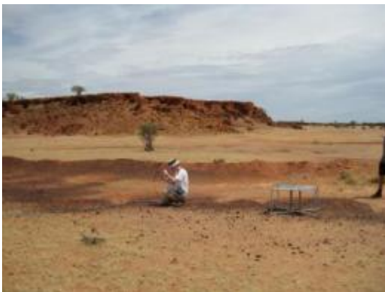
Bowman attaches the coaxial cable to the first-stage analog receiver electronics (the receiver is the metal box). The cable runs from the computer housed inside the hut to the receiver, which is located under the antenna. Credit: Judd Bowman
