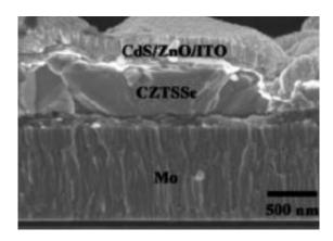
This image shows a cross-section of a CZTSSe thin film solar cell. The film exhibits densely packed grains, which leads to a high efficiency. Image credit: Qijie Guo, et al. ©2010 American Chemical Society.
