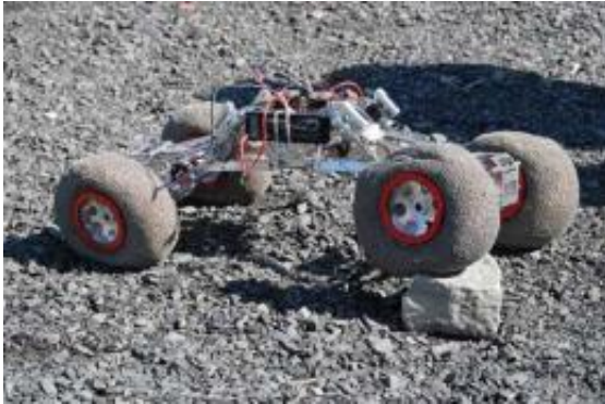
8-inch iRings wheels demonstrating compliance using a rover testbed. / Photo: Brad Jones/Neptec Design Group
