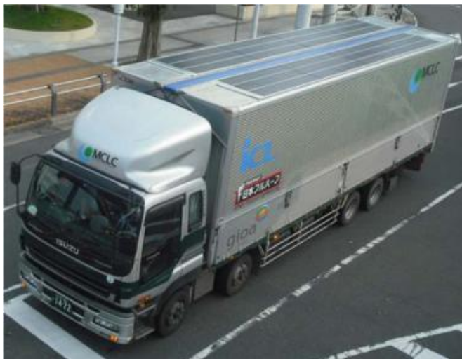
The truck used for a field test of the i-Cool Solar. Image via Tech on.
