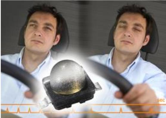
A new infrared light-emitting diode (IR-LED) from the Siemens subsidiary Osram Opto Semiconductors is designed to help recognize the hazardous microsleep that affects motorists. In addition to the IR-LED, this requires a suitable camera with a CMOS sensor. The sensor detects IR light at a wavelength of 850 nanometers, which isn't visible to the human eye, and analyzes the image of the driver that is captured by the camera. And it all takes place unnoticed by the driver - even at night.
