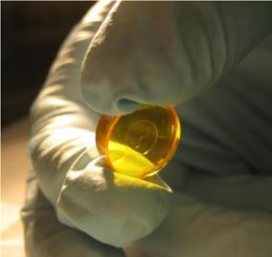
Similar in size and shape to a cough drop, the Apodizing Phase Plate causes light waves coming from a star to interfere with each other, exposing the faint glow of a nearby planet. Shown here is an early version.
