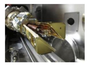
Before the shot: The target is mounted in the cryogenic target positioning device. The two copper-colored arms form a shroud around the cold target to protect it until they open five seconds before a shot.
