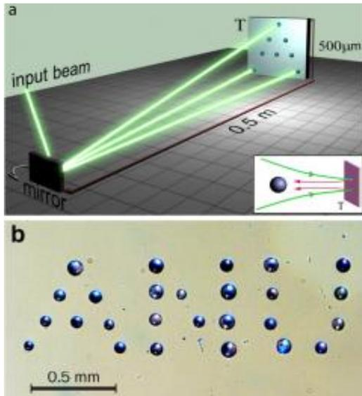
(A) The set-up for transporting particles using optical vortex pipelines. (B) Microspheres form the abbreviation for the Australian National University, having been remotely deposited over a distance of 0.5 meters with a positioning accuracy of 10 micrometers. The microspheres' diameters vary from 60 to 100 micrometers. Image credit: Vladlen G. Shvedov, et al. ©2010 The American Physical Society.
