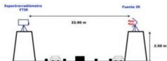
This diagram shows how the system to detect pollution works. Credit: UC3M
