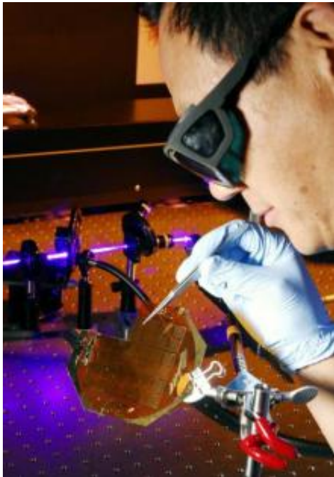
A Georgia Tech researcher manipulates and measures nanodevices based on zinc oxide nanowires fabricated on a flexible polymer substrate. Credit: Credit: Gary Meek
