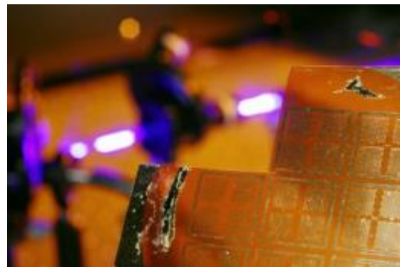
Georgia Tech researchers measure the performance of an array of zinc oxide nanodevices fabricated on a flexible polymer substrate. Credit: Credit: Gary Meek
