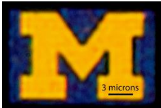
An optical microscopy image of a 12-by-9-micron U-M logo produced with this new color filter process. Credit: Jay Guo
