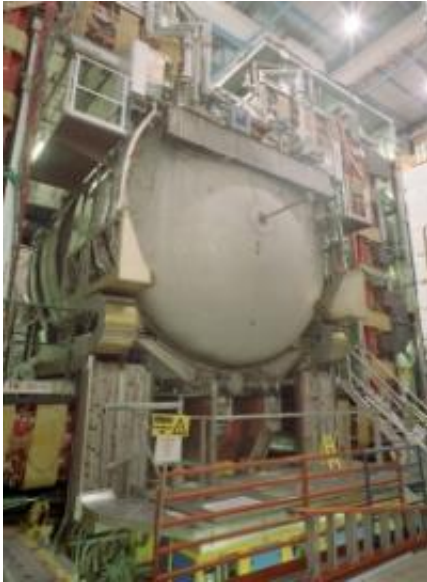
DZero detector showing the large liquid argon calorimeter. (Credit: Fermilab)
