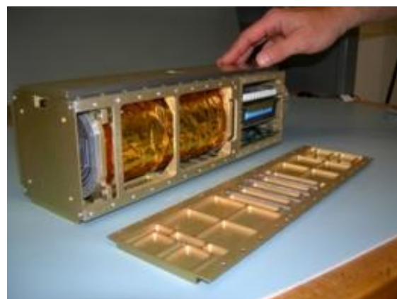
The insides of a standard nanosatellite. Credit: NASA Ames
