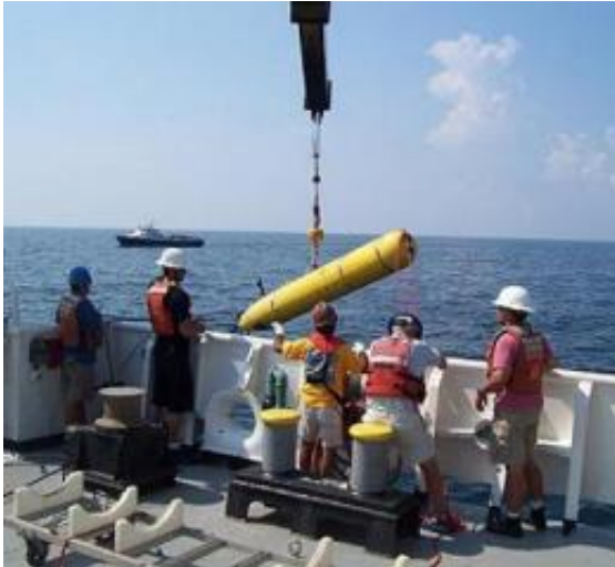
An autonomous underwater vehicle from the Monterey Bay Aquarium Research Institute (MBARI) being launched from the NOAA Ship Gordon Gunter in the Gulf of Mexico Credit: Yanwu Zhang © 2010 MBARI
