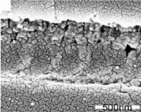
SEM showing surface roughness of the fs-laser machined nanochannel. Image credit: *Nature Nanotechnology*, doi:10.1038/nnano.2010.81.
