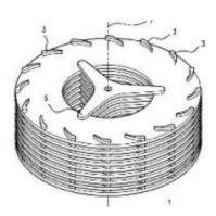
(Left) The bladeless wind turbine, and (right) the stack of disks which rotate and are connected to a shaft. Image credit: Solar Aero.
