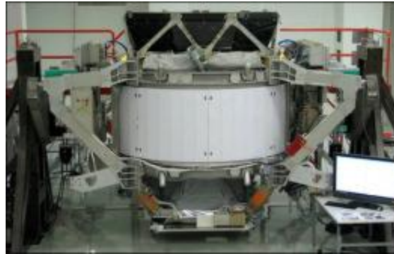
AMS removed from storage facility and being tested.
