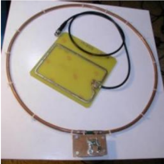
This is a home-made, extended-range RFID antenna made from cooking gas copper pipes in Professor Wool's lab. Credit: AFTAU
