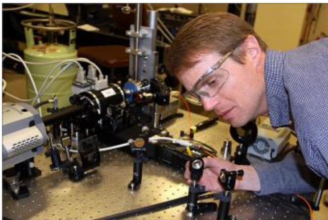
NREL Senior Scientist Brian Flugel adjusts mirrors to set up an experiment aimed at testing the quality of a green LED. Credit: Bill Scanlon
