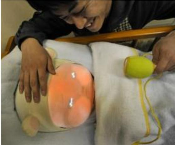
An engineering student soothes Yotaro, a robot which emulates a real baby at Tsukuba University in Japan. Yotaro's face, made of soft translucent silicon with a rosy hue, is backlit by a projector connected to a computer to simulate crying, sneezing, sleeping and smiling, while a speaker can let out bursts of baby giggles.
