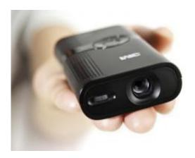
New, particularly high-performance light-emitting diodes (LEDs) from Osram make it possible to build mini projectors. These LEDs produce enough light to project images measuring over one meter in diagonal on a wall. The small, efficient light sources are the key components of a new pocket projector from 3M. Measuring just twelve by six centimeters, the projector fits easily in any handbag and can be connected to cell phones, laptops, or cameras.
