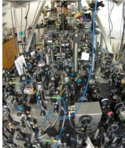
The mirrors and lenses on this optical bench prepare six lasers to capture cold atoms in the atom interferometer (at rear). (Damon English/UC Berkeley)
