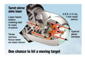
This airborne laser mounts to the front of a special military 747 jumbo jet.
