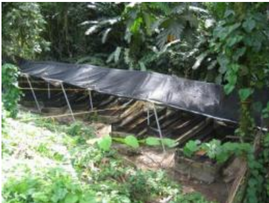
This photo shows the replicate, artificial streams used in the experiments. In total, 16 such streams were used. Credit: Ronald Bassar, UC Riverside.
