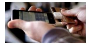
By plugging a small piece of hardware into a phone's audio jack, users can swipe credit cards and transfer money without the need for an additional machine. Credit: Square.
