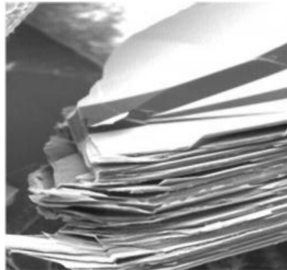
Graphene layers are found in graphite flakes like those from pencil lead. Image: Kirill Bolotkin
