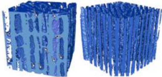
Structure of ice crystals in the presence (left) or in the absence (right) of jumps in the interface. The arrows indicate future defects in the structure. © LSFC 2009
