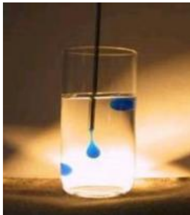
Ionic liquids (in blue) in a beaker of mineral oil. Image credit: John Wilkes.
