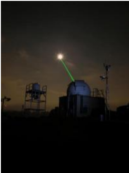
NASA Goddard's Laser Ranging Facility directing a laser (green beam) toward the LRO spacecraft in orbit around the moon (white disk). The moon has been deliberately over-exposed to show the laser. Credit: Tom Zagwodzki/Goddard Space Flight Center
