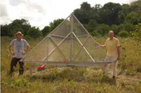
Calibration device near the Cayenne-Rochambeau airport, French Guiana. Corner reflectors such as this one provide a reference signal that can be used to calibrate the airborne radar instrument. Credits: ESA
