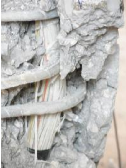
This is a photograph of failed specimen. It is a close-up of a failed GFRP tie and bulged bar. Credit: Antonio De Luca
