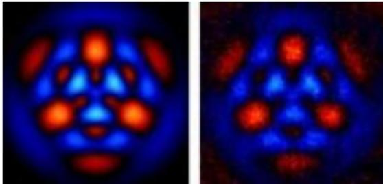
This image represents a quantum state with zero, three and six photons simultaneously. The theory is on left and the experiment is on the right. Image: UCSB.
