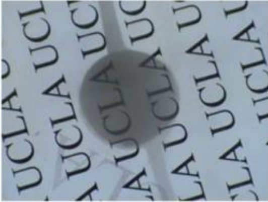
A nanotube film placed over printed "UCLA" lettering prior to stretching. Image courtesy Qibing Pei.
