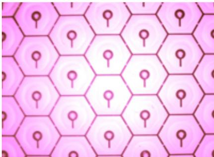
The pixel structure is able to reveal or hide the pigments with high contrast and video speed. The reservoir (center circle) holds the pigment until it is ready to be displayed by application of voltage. Photo credit: Gamma Dynamics LLC
