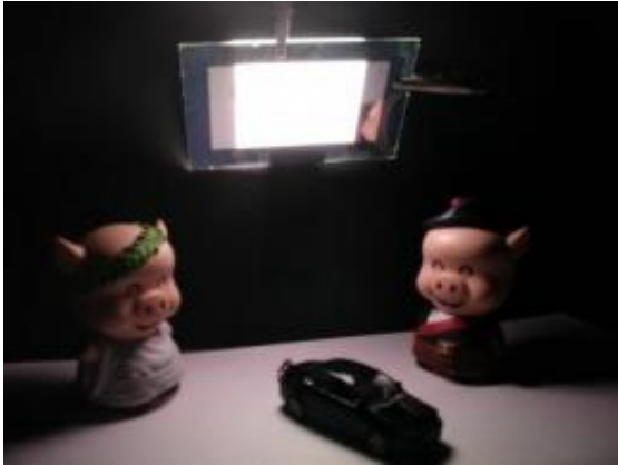
Light produced by a new type of light emitting diode (LED) made from inexpensive, plastic-like organic materials. Photo by Ma Dongge
