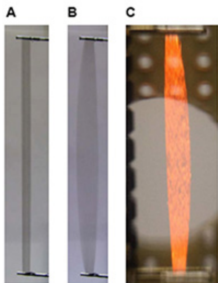
A. An artificial muscle strip with no voltage applied. B. The above artificial muscle strip with 5 kV applied. C. An artificial muscle strip actuated at 1500 K using 5 kV applied voltage.
