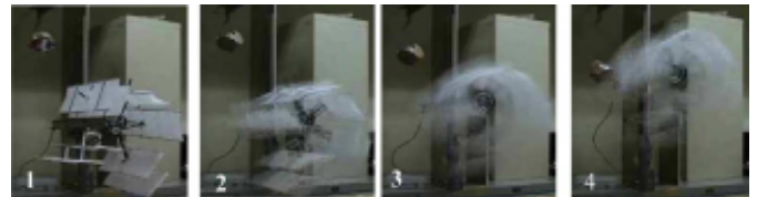
In the flight performance experiment, the cyclogyro robot created enough lift force to fly. Image credit: Naohiro Hara, et al. (c)2009 IEEE.
