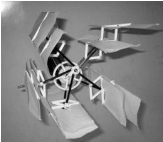
A prototype design of the cyclogyro craft with five pantograph-based variable wing units. Image credit: Naohiro Hara, et al. (c)2009 IEEE.
