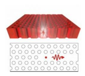
Photonic crystal membrane waveguide with an emitting quantum dot (red dot) in side-view (upper image) and top-view (lower image). An excited quantum dot emits one photon at a time, which is directed into the waveguide with very high efficiency. Image: Peter Lodahl
