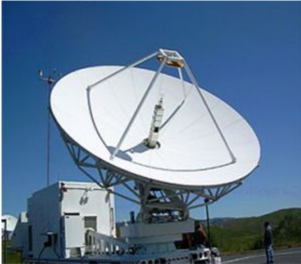
MIT Lincoln Laboratory's LAKaTT satellite terminal, utilized for testing communications over WGS satellites Photo courtesy / MIT Lincoln Laboratory Communications Office
