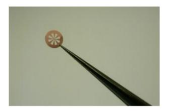
Magnified image of research samples with small holes covered by graphene. One can see light passing through them by the naked eye. Credit: University of Manchester
