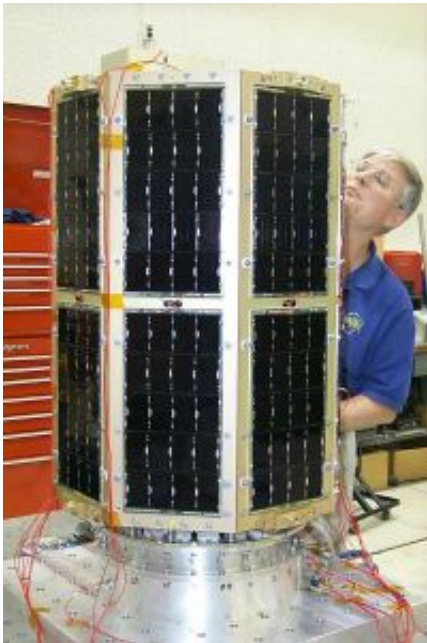
Dr. Billy R. Smith Jr., director of the USNA Small Satellite Program and MidSTAR-1 program manager, inspects MidSTAR-1 for damage after vibration testing at the Naval Research Laboratory. Credit: USNA
