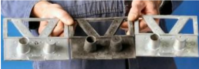
A display of three test castings, which, from left to right, are: 1. As cast (left), 2. Conventional heat treatment (middle), 3. Heat treated using the new procedure (right). Credit: CSIRO
