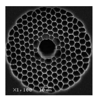
Electron microscope image of the hollow-core fiber. Credit: University of Bath
