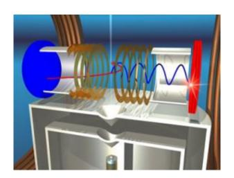
To perform the experiment, a supersonic jet of hydrogen (source at bottom) is ionized by a beam of x-rays from the Advanced Light Source (not shown). The doubly photoionized molecule blows apart, and the protons (red) strike the detector at left while the electrons (blue), trapped in a magnetic field, strike the detector at right. The energy of all the particles and the original orientation of the molecule can be determined from the measured results.
